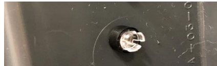
Figure 10. Installed LED Housing
