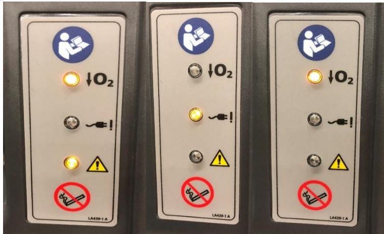
Figure 26. Illuminated Monitoring Lights
